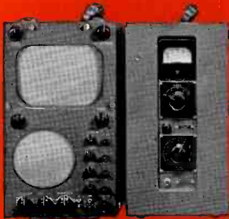
Master control (left) with power supply
