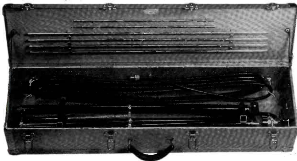
FIG. 2. Accessory Case of the 301-B Equipment. Mounted in the lid are the sections of the extendable dipole. In the lower part of the case are the mounting tripod and the connecting cable.
