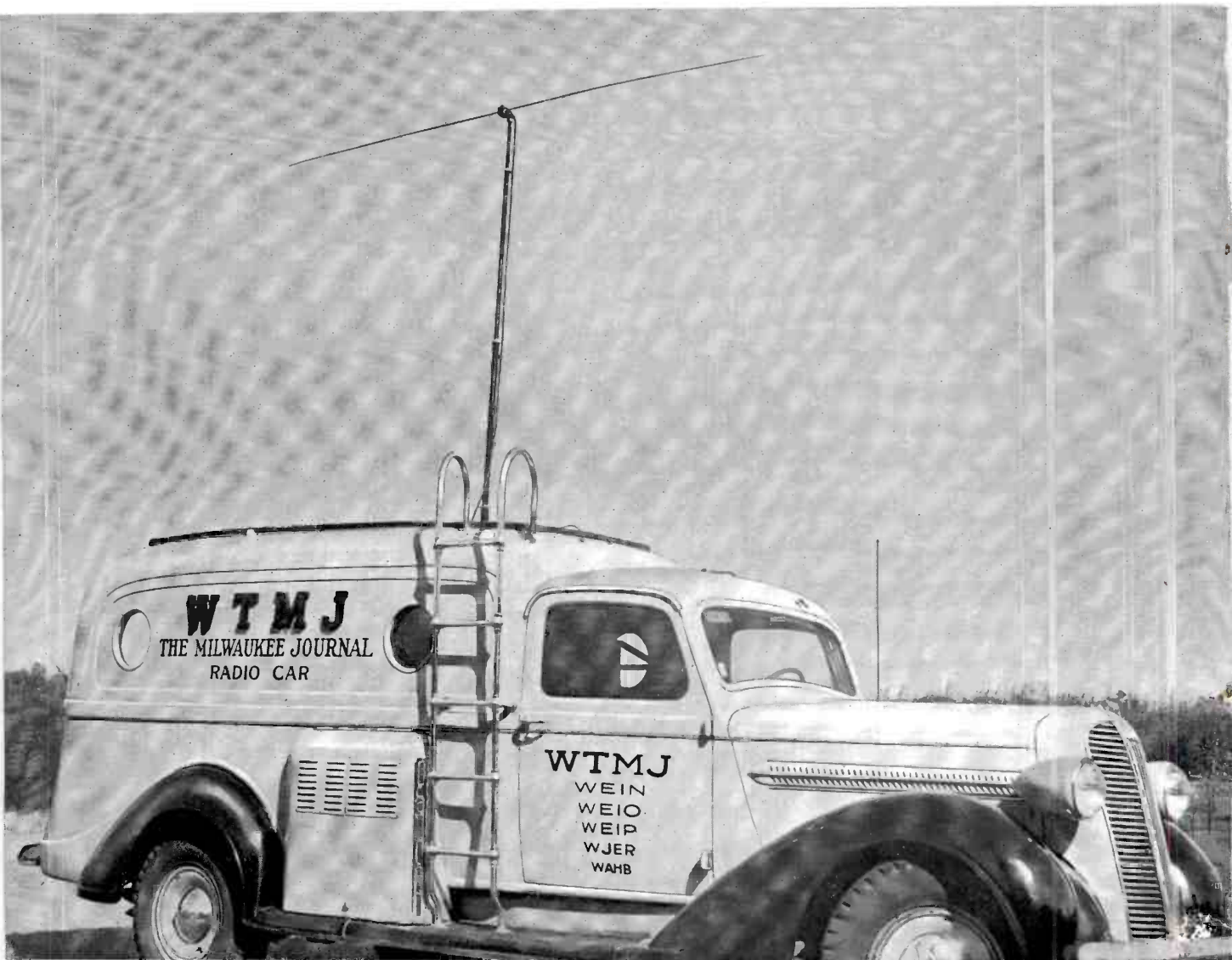
FIG. 1. The field car with the telescopic antenna raised. The antenna pivots on a bearing inside, permitting orientation for maximum signal.
